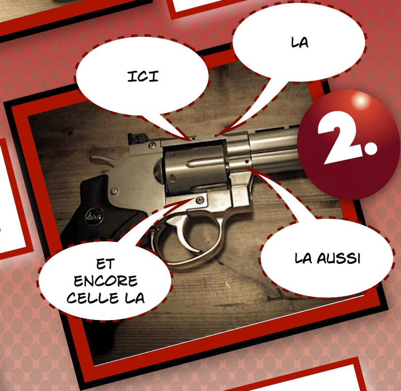
Remove three pins and screw
